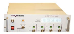
QUAD-EV-C-PSU. A 250W four channel supply with the facility to independently enable and measure output from all channels. This can be used with the QUAD-EV-C source.
