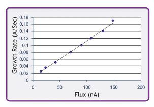
The graph above shows the relationship between deposition rate of molybdenum, as measured by a quartz-crystal monitor and the ion current (flux) measured on the flux-monitoring plate of a QUAD-EV-S source.
